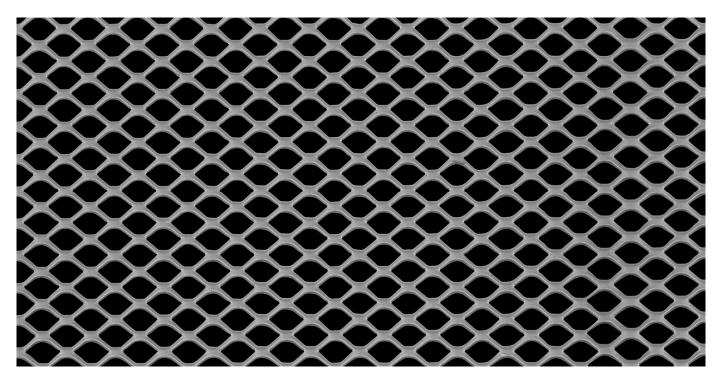
LW Pitch:12.70mmStrand Width:1.30mmSW Pitch:8.50mmThickness:0.90mmWeight:2.16 kg / m2Open Area:69%
